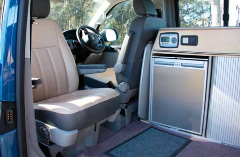
Captain's chairs swivel easily at the touch of two levers and opens up the interior.
